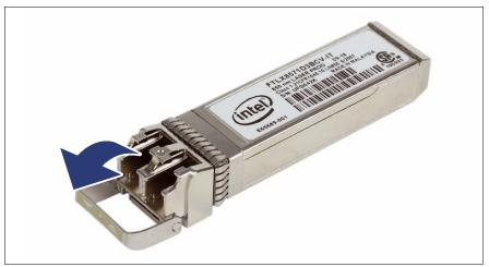
Figure 46: Unlatching the locking bail
